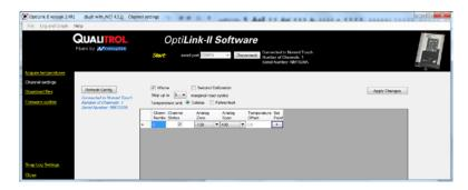
Once you have made the required changes to the displayed matrix of parameters, you must upload these changes by clicking "Apply Changes".
