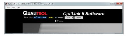
This application requires that you know which serial com port or which IP address will be used by OptiLink-II. The COM port selector will only list the currently available ports on your Windows; this is the same list of available ports you would view in your Windows Hardware Device Manager. With the Nomad-*Touch*, the IP connection option is not available, as the Nomad-*Touch* does not support an Ethernet link. Click the Connect button. The following window will open:
