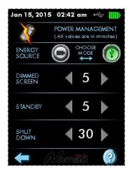
From this screen, you can optimize the battery use parameters (when connected and not connected to USB). Note: "-" means "never".
