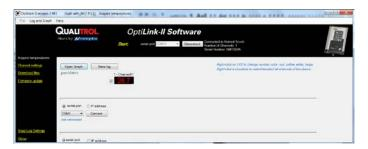
This window also includes a "Graph" button, which will open an additional window that will show a trend graphic for all previously selected channels (channel selection should be made prior to opening this second window). See section 8.2.2 for more information.
